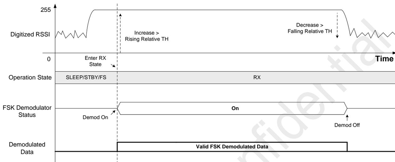
**Figure 33. Entering RX with Signal Being Transmitted**
