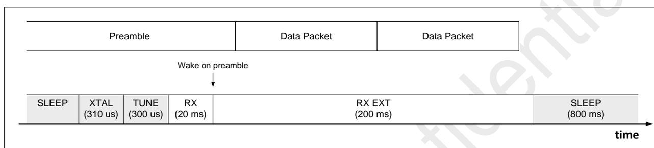
**Figure 23. Preamble Wake-On Operation with Preamble Detected**
