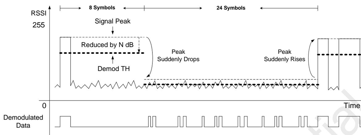
**Figure 29. OOK Demodulation Using Peak - N Threshold, with Peak Drop Off**
