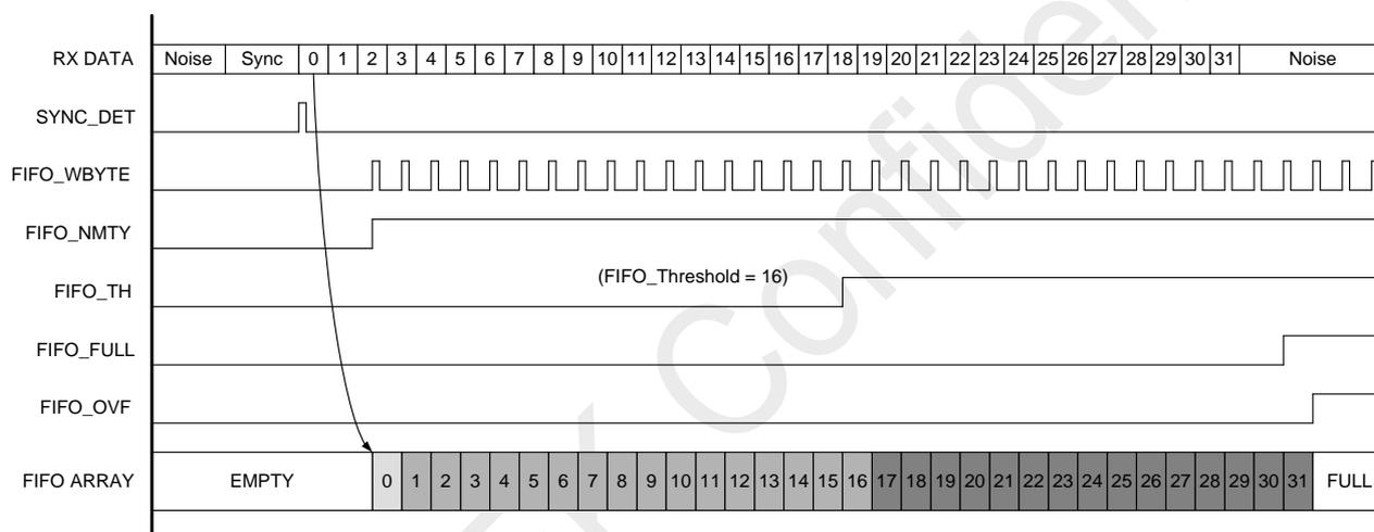
**Figure 40. FIFO Interrupts Timing Characteristics**
