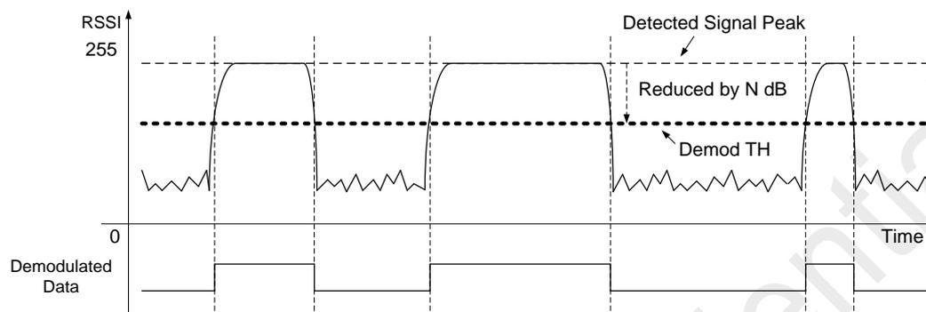
**Figure 28. OOK Demodulation Using Peak - N Threshold**
