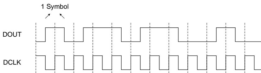
**Figure 38. Timing Characteristic of DOUT and DCLK**
