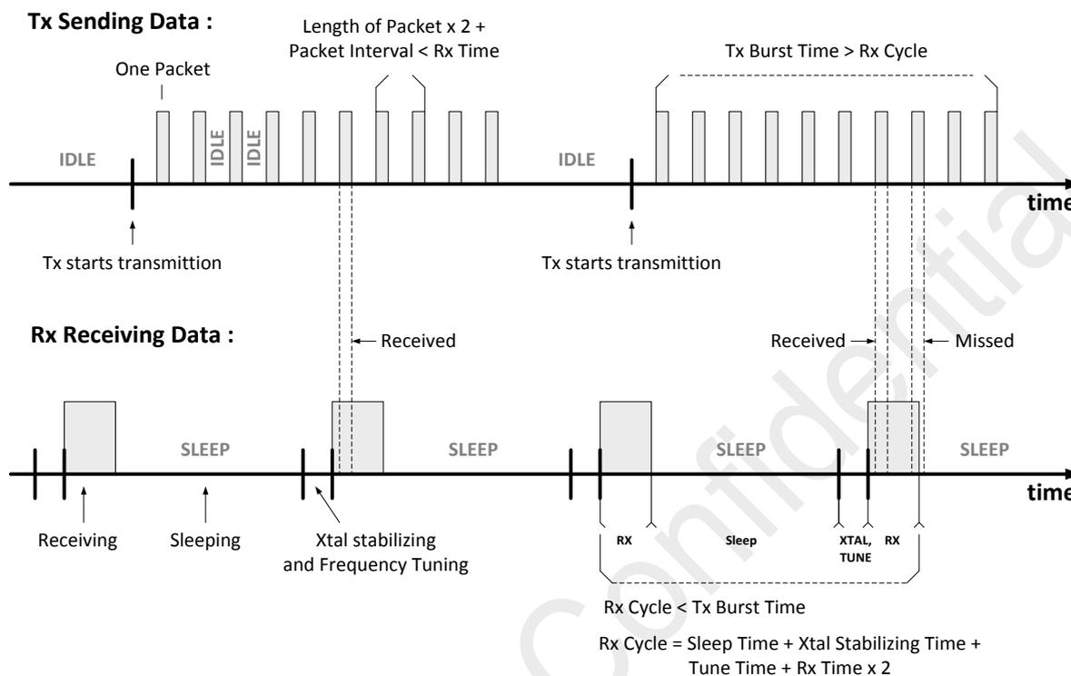
**Figure 20. Tx and Rx Relationship of Precise Configuration**
