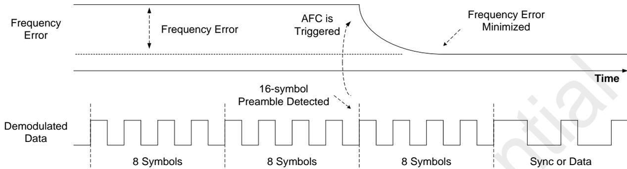
**Figure 35. AFC Timing Characteristics**
