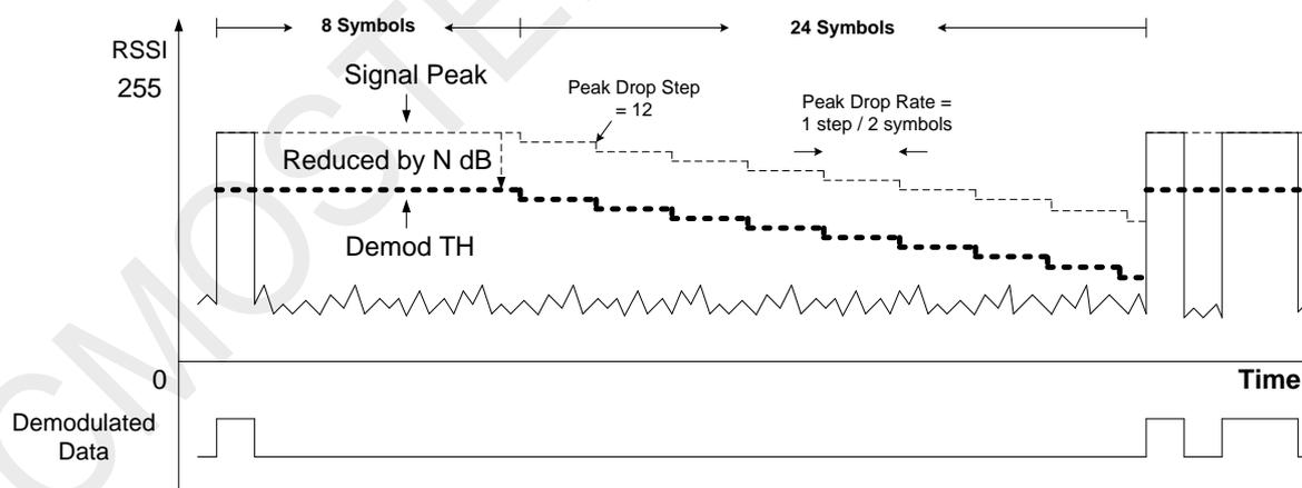
**Figure 30. OOK Demodulation Using Peak - N Threshold, with Peak Drop On**
