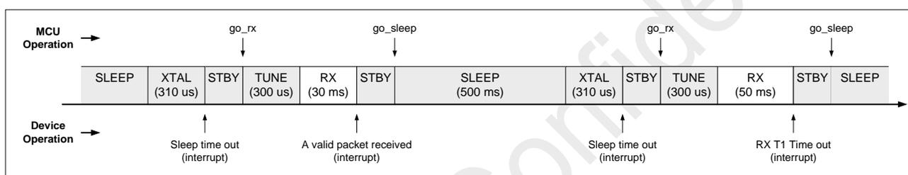
**Figure 9. Fixed Duty + Early Exit Operation**
