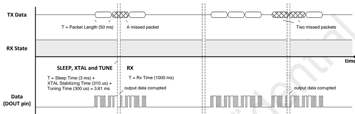
**Figure 19. Tx and Rx relationship of Easy Configuration**
