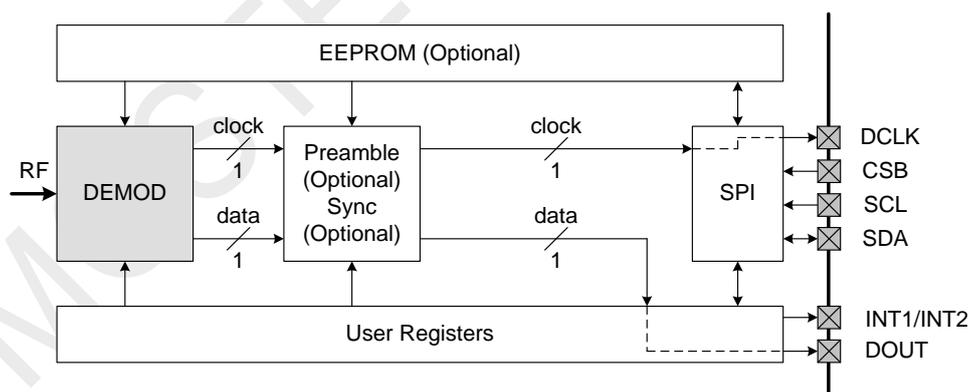
Figure 37. Data Path of Direct Mode
