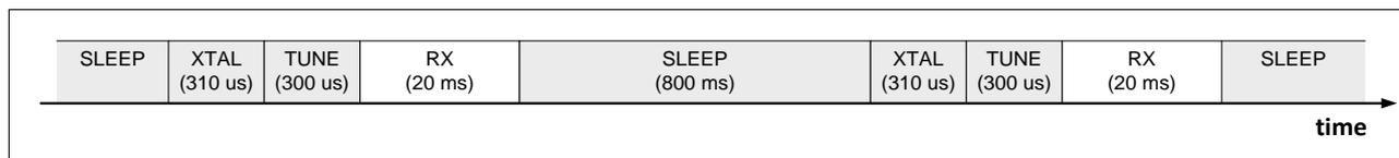
**Figure 22. Preamble Wake-On Operation without Preamble Detected**
