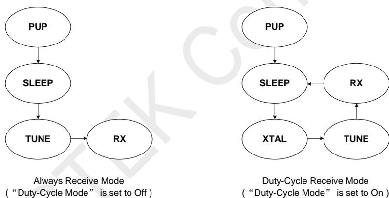
Figure 16. Radio Operation with Duty-Cycle Mode On and Off
