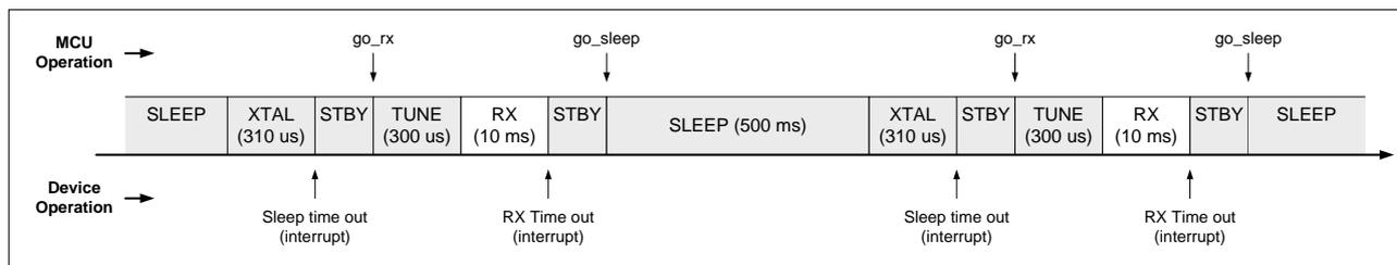
Figure 10. Wake on Preamble without Valid Signal Operation
