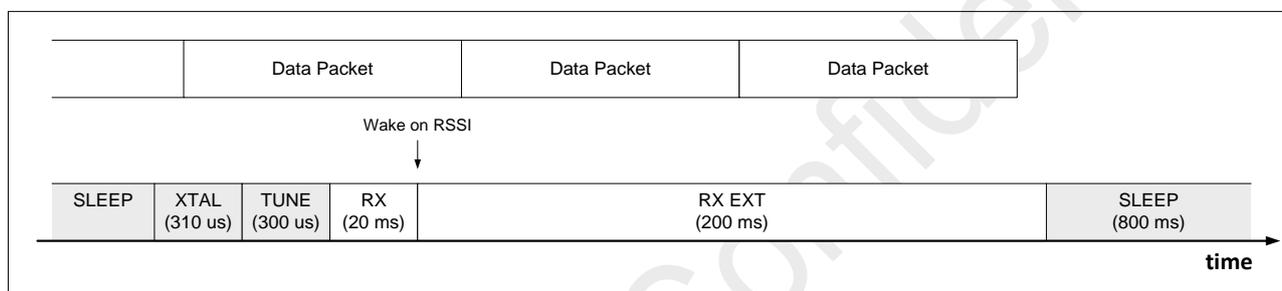
**Figure 25. RSSI Wake-On Operation with RSSI Detected**
